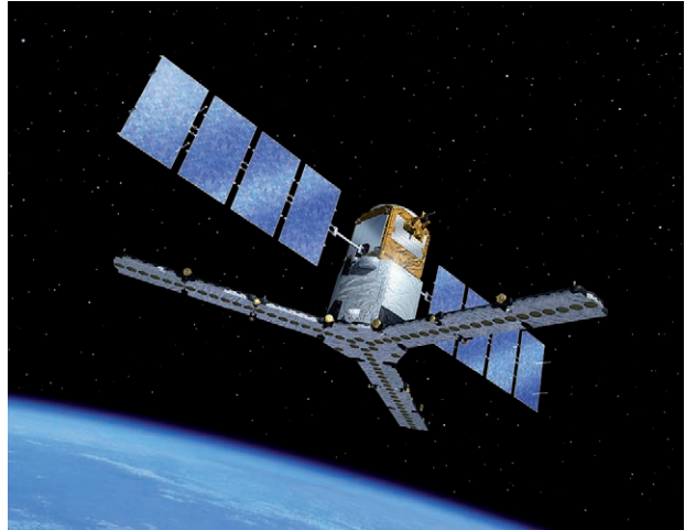
FIG. 1. – Artist's view of SMOS in flight configuration. The lower part shows the MIRAS radiometer with its 69 antennas along the three arms (credit: ESA-AOES Medialab).
