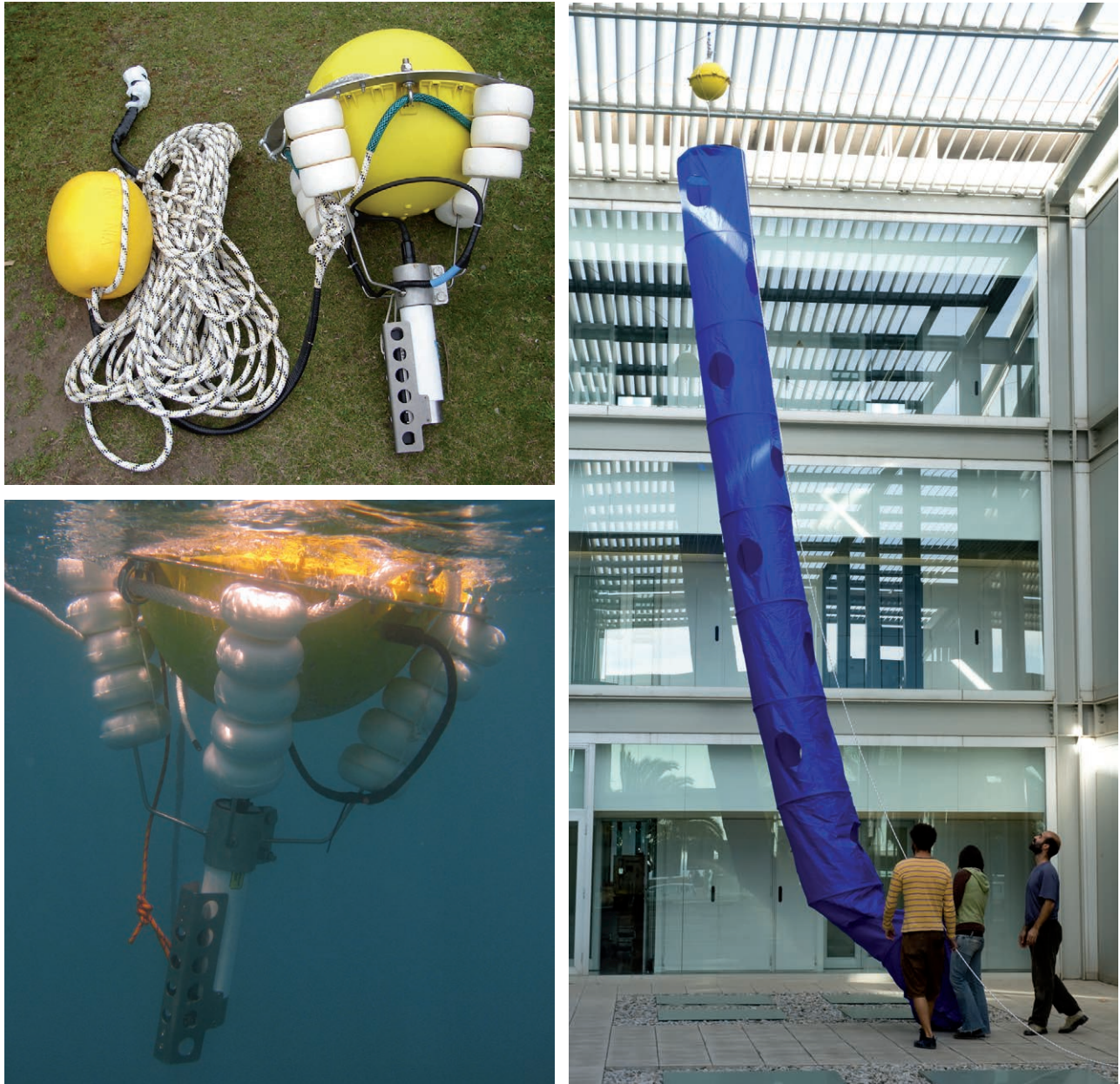
FIG. 6. – Prototype of surface drifting buoy designed by SMOS-BEC to measure salinity at 50 cm below the surface. It carries a high quality temperature-conductivity recorder (SeaBird SM37) and a 10-m-long holy-sock drogue to ensure drift by surface currents and not by wind or waves (credit: J. Salvador, L. Lizarazu, M. Gasser).
