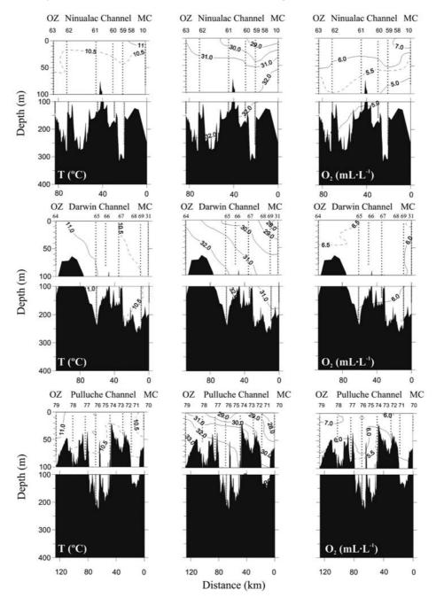
FIG. 3. – Vertical distribution of temperature, salinity, and dissolved oxygen in the Ninualac, Darwin, and Pulluche channels. OZ: Oceanic Zone, MC: Moraleda Channel.
