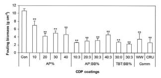
Fig. 3. – Comparison of total fouling biomass estimated on CDPcoated panels exposed for three months to waters of Ayajin harbour, South Korea. Means are compared with control by one-way ANOVA followed by Dunnett's test (\*p<0.05; \*\*p<0.01).
