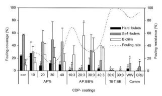
Fig. 2. – Comparison of coverage (%) of major components of fouling assemblages on CDP-coated panels exposed for three months to waters of Ayajin harbour, South Korea. Means are compared with control by one-way ANOVA followed by Dunnett's test (\*p<0.05).
