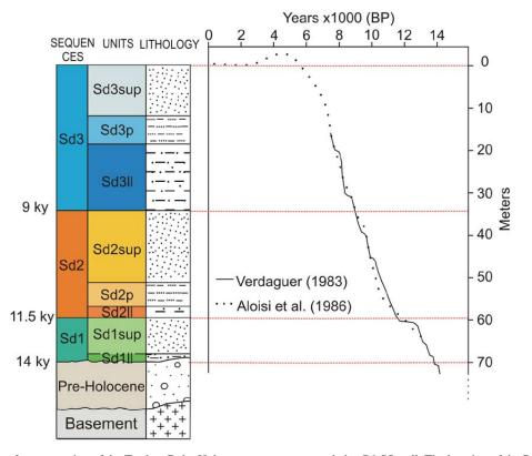
Fig. 11. – Standard reference section of the Tordera Delta Holocene sequences recorded at P6-S5 well. The location of the P6-S5 well can be seen in Figure 2.
