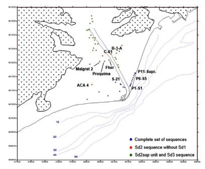
Fig. 2. – Situation Map of the 50 wells and piezometers on the Tordera Delta plain under study. The colours indicate the different types of well classified as a function of the number of stratigraphic sequences and units present.
