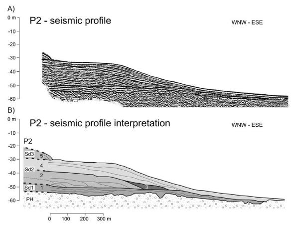
Fig. 5. – Sequence boundaries and internal reflection configuration from profiles P1 to P4 (see Fig. 1 for situation), including seismic reflection patterns (aggradation) and terminations (toplap, downlap and coastal onlap).
