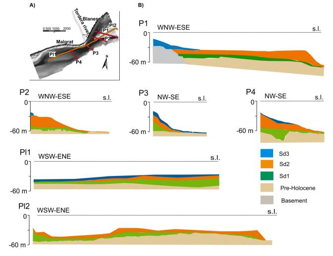
Fig. 7. – A, image of slope gradients (modified from UB-Pridesa in Alfaro 2011) and situation of different seismic profiles: P1-P4 and PL. B, interpretation High-resolution seismic profile (see Fig. 5) showing three sequences Sd1, Sd2 and Sd3, PH and basement of the Tordera prodelta and inner shelf. A large paleochannel on the erosive base of Sd1 can be distinguished on P4.
