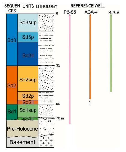
Fig. 3. – Standard lithological reference section and depths (comprising all units) of the Tordera Delta Holocene sequences, as recorded at the P6-S5 well. The map in Figure 2 shows the three well types as a function of the sequence content: pink contains all the sequences (as in P6-S5 well), orange does not contain Sd1-Sd2ll (as in ACA-4 well), and green only contains Sd3 and Sd2sup sequences (as in B-3-A well).
