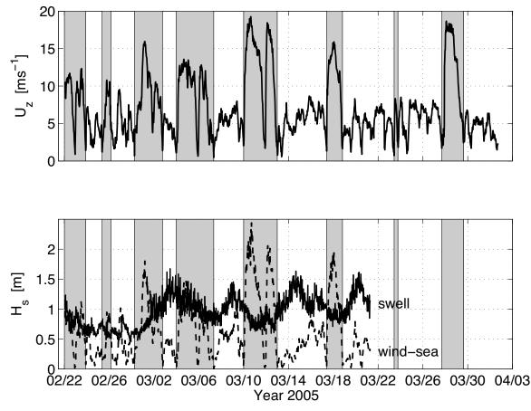
FIG. 2. – Time series of mean wind speed (top), significant wave height of swell (bottom, solid line), and wind sea (bottom, dashed line), as observed at the ASIS buoy during the IntOA experiment. Shaded areas denote the Tehuano events.
