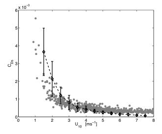
FIG. 10. – Swell-related drag coefficient  $(C_{D_s})$  computed from the wind velocity spectrum coherent with the waves (circles) as a function of wind speed. Diamonds are the mean  $C_{Ds}$  computed from the relationship of Pan *et al.* (2005) for wind increments of 1 m s<sup>-1</sup> and error bars are two standard deviations.
