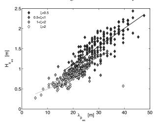
FIG. 8. – Wind sea significant wave height,  $H_{s_{WS}}$ , as a function of wind sea wave length,  $\lambda_{ws}$ . Colours denote different swell importance parameters,  $\zeta$ ; ranges and lines are the linear fit in each range.
