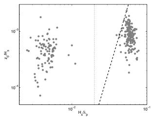
FIG. 9. – Dimensionless surface roughness as a function of the wave steepness. Lines are the parameterization of Taylor and Yelland (2001) (dashed) and the limit suggested by Drennan *et al.* (2005) (dotted).
