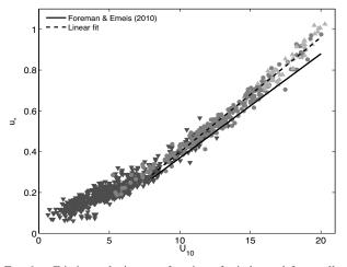
FIG. 6. – Friction velocity as a function of wind speed for swelldominated conditions (down triangles), wind sea-dominated conditions (circles), and the subset of strongly wind sea-dominated conditions (up triangles). Lines represent the linear fit (dashed), and the parameterizations of Foreman and Emeis (2010).
