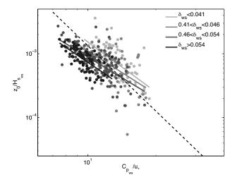
FIG. 7. – Dimensionless surface roughness as a function of the wind sea wave age. Colours denote different wind sea steepness,  $\delta_{ws}$ , ranges and lines are the logarithmic fit for different wind sea steepness ranges (solid) and the parameterization of Drennan *et al.* (2003) (dashed).
