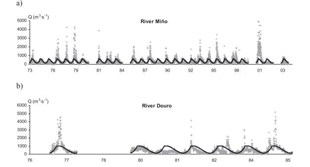
FIG. 4. – Plots showing the high inter-annual river discharge variability and the error-fitting with climatological values. River discharge data corrected as explained in Material and Methods (grey dots) is compared to the estimated climatological value from the Results section (black line). The complete available time series is plotted in the River Miño (a); nevertheless, only data estimated from the Rio Mau station are plotted in the River Douro (b) to avoid a very long time series.
