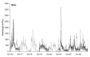
FIG. 6. – Mean daily discharge at the mouth of the River Miño directly estimated from gauge records at *Foz do Mouro* station (black line), estimated from runoff observed in the River Douro (thick gray line) and from precipitation (thin gray line).
