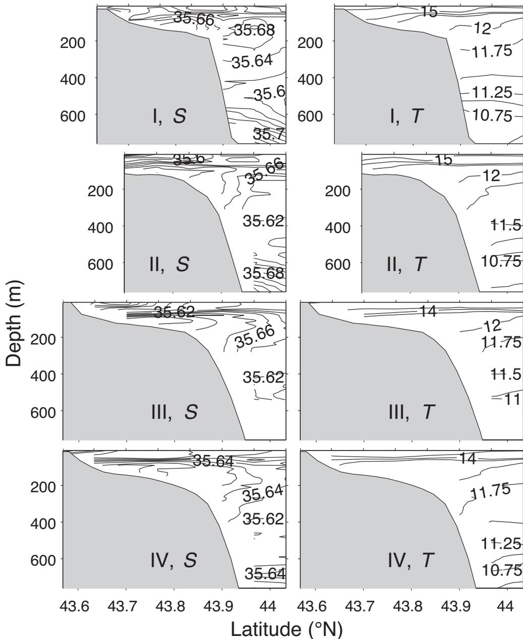
FIG. 10. – Salinity (*S*, left) and temperature (*T*, right) vertical sections during the ESE00506-I cruise as a function of latitude. Sections are numbered from west (upper row) to east (lower row) as shown in Figure 2A.
