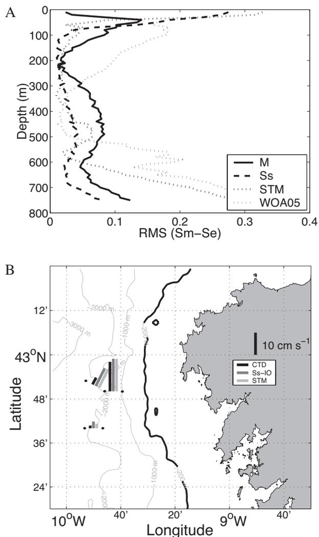
FIG. 14. – A, rms of the difference between measured and estimated salinity (see text for details); B, surface geostrophic velocity during the FINISTERRE-2006 exercise estimated with CTD data and with our best polynomial coefficients ( $Ss-IO$ ).
