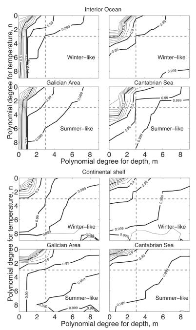
FIG. 8. – Upper: R2a contour lines for Galician Area and Cantabrian Sea corresponding to the winter-like and summer-like seasons in the interior ocean, as a function of polynomial degrees. Lower: same as before, but on the continental shelf. Gray dashed lines indicate the degrees of the polynomial fit finally used.
