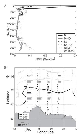
FIG. 11. – A, rms of the difference between measured and estimated salinity for six cases indicated in the legend (see text for details); B, surface geostrophic velocity during the GIJON-2006 exercise estimated with the CTD data, with our best polynomial coefficients (Ss-IO) and with STM case.
