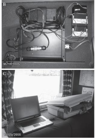
FIG. 1. – A, schematic diagram of the XBT acquisition system adapted to work autonomously; B, detail of the aerial amphenol connectors to the battery pack; C, the suitcase containing the desk system and the laptop used in the exercises.
